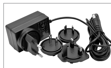
Universal power supply included 24 VDC/1 A - 100÷240 VAC input 3 m cable length
