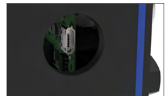
MICRO USB FOR PC CONFIGURATION
